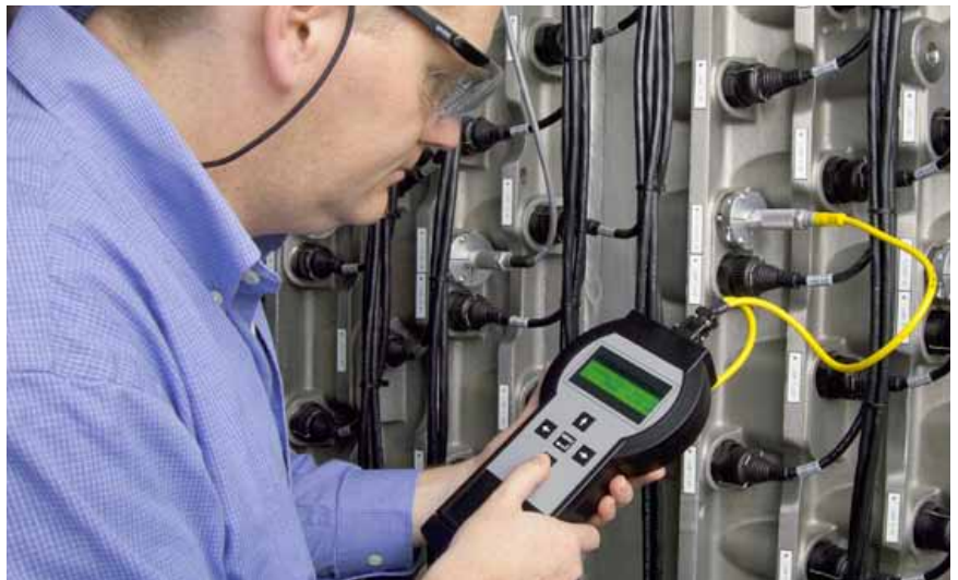
The hand-held UV Intensity sensor monitor allows operators to quickly and easily measure duty and reference sensor calibration.
