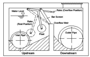
Figure 1 TRU-RAKE Operational diagram
