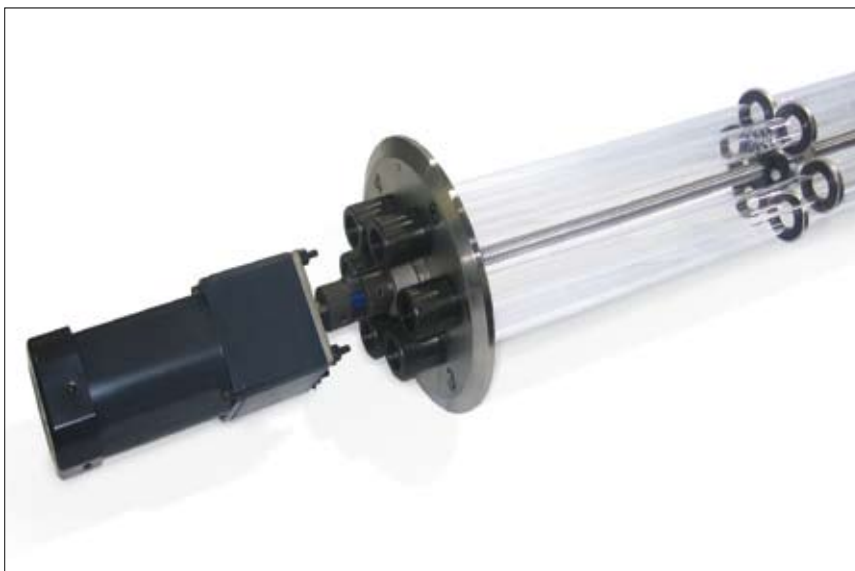
The optional wiping systems reduce maintenance costs. Operators have a choice of the manual system that is operated by hand, or motorized system (shown above) which can be programmed to wipe automatically at preset intervals.
